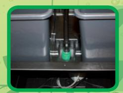
**5.** Fit down-pipe of delivery assembly to adaptor on outlet end of pump. Place pump in position and secure far end of delivery assembly in position with cable tie.
