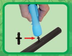
3. Screw the black top from the tool. Push the black nipple on the tool and push them into the tube.
