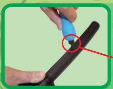
2. Use the blue tool, to make a hole in the tube.
