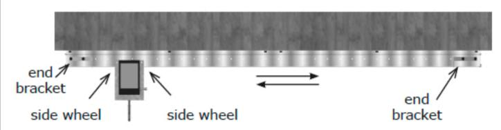
After you finish installed motor, screw in the other end bracket. Plug it in to start, drive motor will start moving. When it moved to the end, the side wheel will touch the "end bracket" then it pause for whatever time you configure earlier and then it continues moving other direction.
